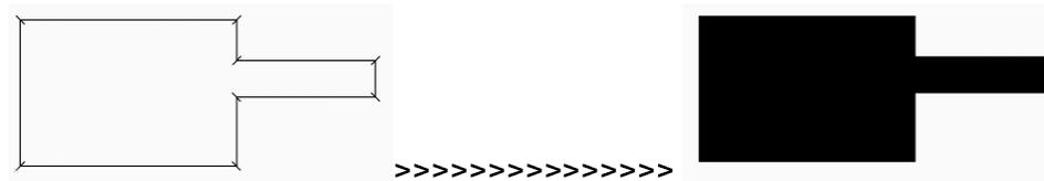
**Possibility 3:** A continuous closed line surrounds one or more other lines. The differences between these surfaces defines the remaining copper surface.
